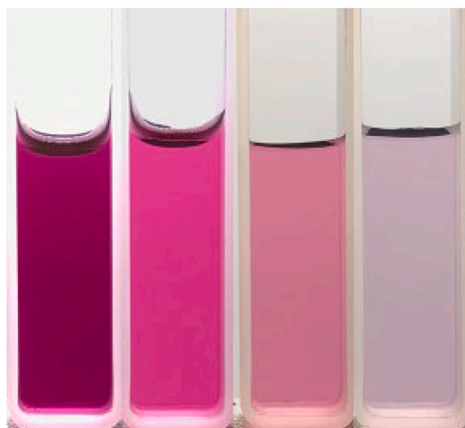
Fig. 3. Transmission light color of gold nanoparticle solutions before centrifugation and after the first, second, and third centrifugation, shown from left to right.
