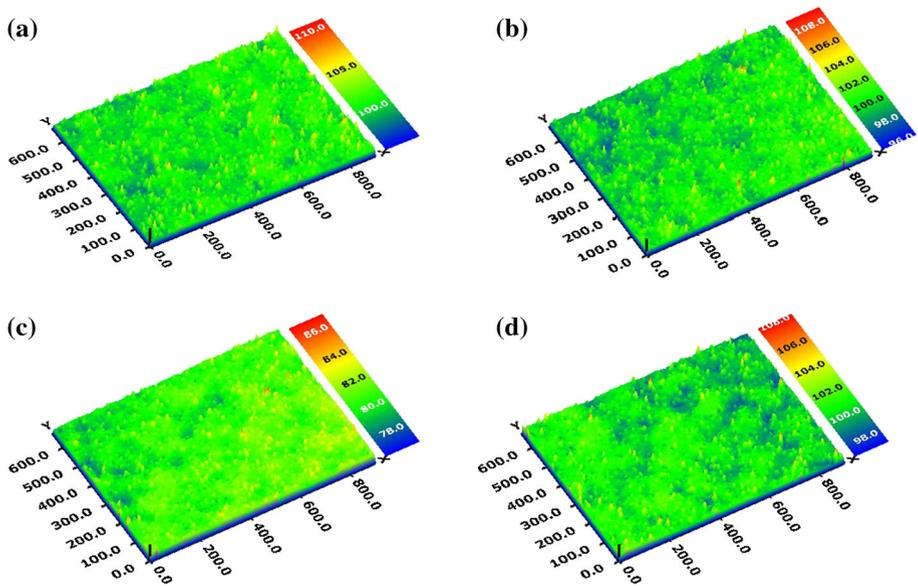
**Fig. 4** Surface morphologies of: **a** bare Ch-LC layer, **b** one-step ITO layer (100 nm), **c** two-step ITO layer (30 + 70 nm), and **d** two-step ITO layer (50 + 50 nm)
