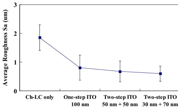
**Fig. 5** Average surface roughness ( $S_a$ ) values of various samples as measured using three-dimensional microscopy
